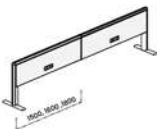
2 Desks Length: 3000 / 3200 / 3600 [mm] Height: 770 [mm] Thickness: 75 [mm]
